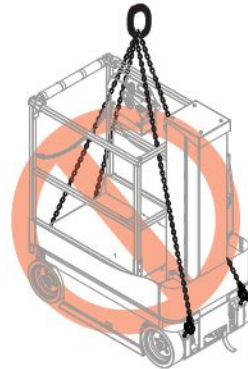
Figure 3-12. Inappropriate Lifting Method
